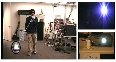
Figure 5. Left is a camera phone being neutralized by our system (notice the neutralizing light beam over the lens). Top right is the camera view neutralized by the system and bottom right is the camera view when the camera is permitted to capture.
